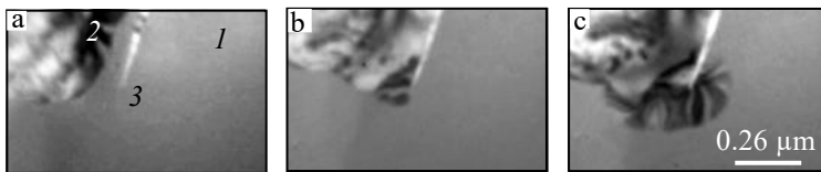
Figure 5.16 - Bypassing the obstacle by the crystallization front. Microphotographs correspond to time points t that have passed since the beginning of filming: (a) t = 0 s; (b) t = 0.42 s; (c) t = 1.40 s; 1 – amorphous phase; 2 – disk-shape \text{Cr}_2\text{O}_3 crystal; 3 – needle-shape \text{Cr}_2\text{O}_3 crystal [110]
